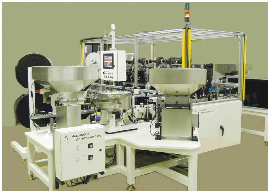
Designed and built by Automation Development for five-piece pump assembly, this machine produces 100 assemblies per minute. The automation and assembly equipment designed and manufactured at Automation Development is complex, in many cases requiring over 6,000 parts. Eliminating outsourcing has given them control over the project costs and schedules.
